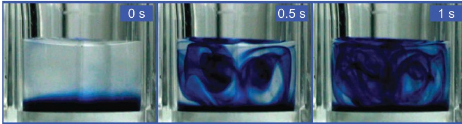
Fig. 14 Surface acoustic wave (SAW) induced mixing in one well in a 96-well plate. The well diameter is approx. 6 mm. Figure taken from Wixforth. 73
