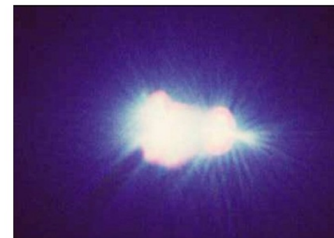
Figure 71. Colour photograph of the light emitted by a trapped, positionally unstable bubble. Long exposure. (Courtesy of R Geisler.)
