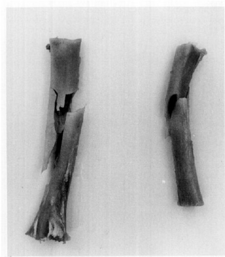
FIG. 4. Complete fractures of the bones occurred after 10,000 shock waves at maximum energy density ( 0.60 \text{ mJ/mm}^2 ). This photograph shows two femurs.
