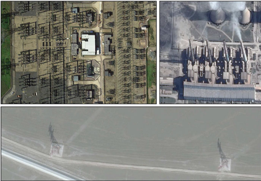
Fig. 1 Images of power system components from GIS. Top left: transmission substation, top right: power plant, bottom: power lines
