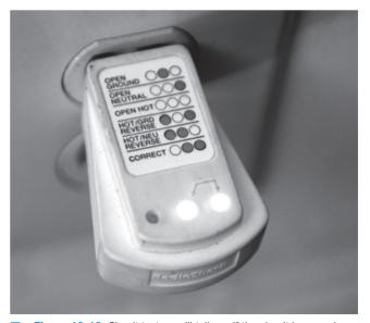
Figure 18-13 Circuit testers will tell you if the circuit is properly wired with a "hot," a "return," and a ground. It's not uncommon to find improperly wired outlets.
