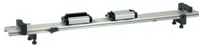
Figure 4.2 Low-friction track and carts used in the experiments described in this chapter.
