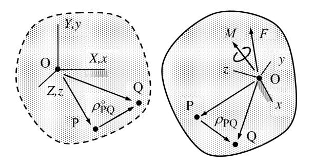
The primary unknowns are u, v, w,  $\phi$ ,  $\theta$ ,  $\psi$  of the translation point. Body may translate and rotate but distance between any two points P and Q is constant. Mathematically, e.g.,  $\vec{u}_{\rm Q} = \vec{u}_{\rm P} + \vec{\theta}_{\rm P} \times \vec{\rho}_{\rm PQ}$ . Forces acting on the body can be represented by a force-moment pair.
