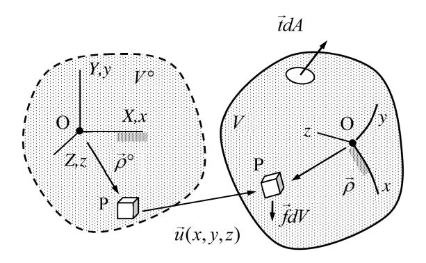
The primary unknowns are u(x,y,z), v(x,y,z), w(x,y,z),  $(\phi(x,y,z), \theta(x,y,z), \psi(x,y,z))$ . Material elements may translate, rotate, and deform. In short, for points P and Q of an element  $\vec{u}_Q = \vec{u}_P + \vec{\theta}_P \times \vec{\rho}_{PQ} + \vec{\rho}_{PQ} \cdot \vec{\varepsilon}_P$ . Displacement follows from stress-strain relationship (generalized Hooke's law) and equilibrium of material elements.
