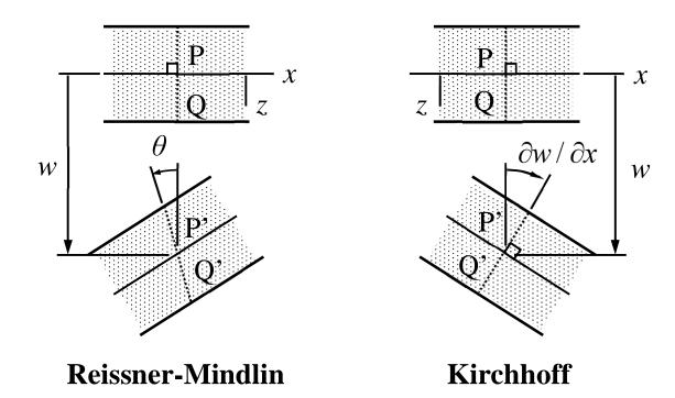
The primary unknowns are u(x,y), v(x,y), w(x,y),  $\phi(x,y)$ ,  $\theta(x,y)$ ,  $\psi(x,y)$ . Line segments perpendicular to the mid/reference-plane remain straight in deformation (Reissner-Mindlin) and perpendicular to the mid-plane (Kirchhoff). Mathematically  $\vec{u}_Q = \vec{u}_P + \vec{\theta}_P \times \vec{\rho}_{PQ}$ . Normal stress  $\sigma_{zz}$  is negligible.
