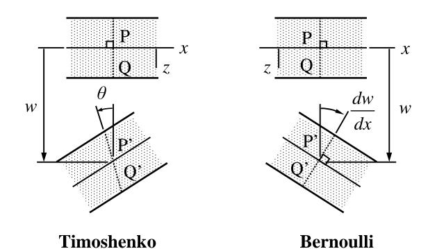
The primary unknowns are u(x), v(x), w(x),  $\phi(x)$ ,  $\phi(x)$ ,  $\psi(x)$ . Normal planes to the (material) axis of beam remain planes (Timoshenko) and normal to the axis (Bernoulli) in deformation. Mathematically  $\vec{u}_Q = \vec{u}_P + \vec{\theta}_P \times \vec{\rho}_{PQ}$ . Transverse normal stress is negligible, i.e.,  $\sigma_{yy} = \sigma_{zz} \ll \sigma_{xx}$ .
