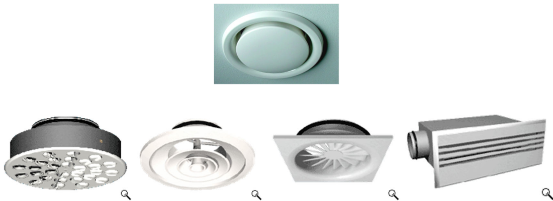
Fig. 7.5.1 Top exhaust air valve. The shape of exhaust air valves varies less than that of supply air valves. The most typical supply air valves look pretty much the same as the exhaust air valve in the picture. If the supply air is to be directed more efficiently, diffusers are used, for example. At the bottom there is a nozzle, cone, vortex and wall diffuser (Fläkt Woods Oy 2006).
