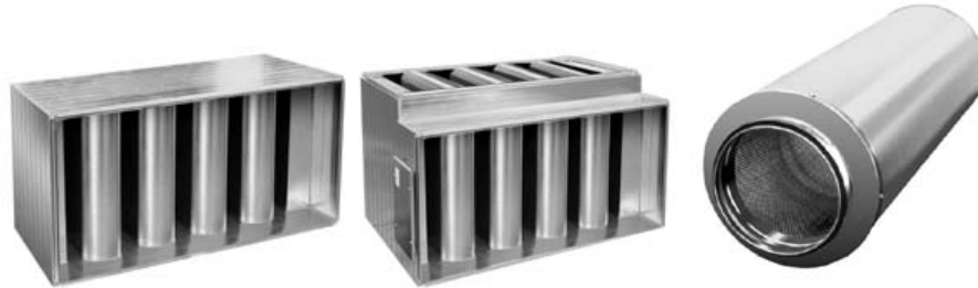
Fig. 7.7.1. (a) Straight lamella silencer, (b) lamellar silencer with 90° angle, (c) cylindrical duct silencer. The lamellas are an absorbent material. In a direct muffler, the absorption material is on the walls. Usually, the absorption material is protected, for example, with perforated sheet metal to prevent the absorption material from tearing in the air flow or sweeping the ductwork.
