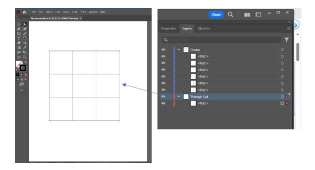
With the blade cutters program it is possible to define the lines into crease and cut, but the process is much more quicker and easier if it is done in advance.
