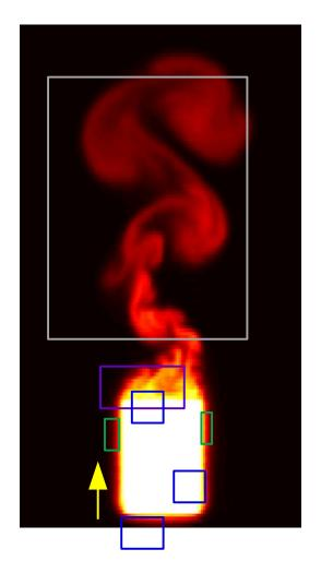
Step 5: fluid rises constantly and the hot air is "self-transported" away from the object in a plume which poses fluid dynamical structures (e.g. vortices, turbulence)
