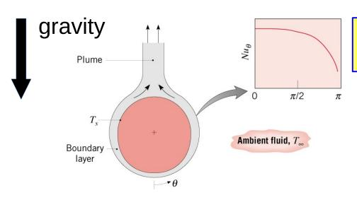
$$Ra = \frac{g \beta (T_s - T_{\infty}) L^3}{v \alpha} = \frac{Buoyancy force}{Viscous force}$$
