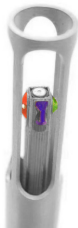
Figure: Measurement of 3D intensity with 3 velocity sensors directed at XYZ axes, and a coincident pressure sensor. Scale: centimeters.
