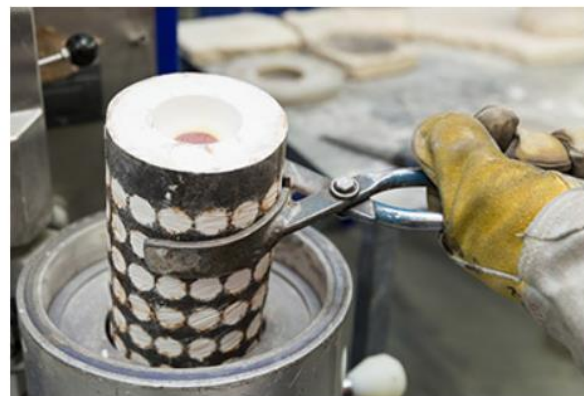
The wax has been melted off from the cylinder and replaced with molten metal.
