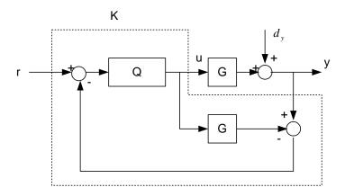
Note that in addition to the reference r a disturbance signal  $d_y$  is modelled to enter at the output of the process. By using the IMC design discussed in the lectures analyse the response to step inputs at r and  $d_y$ .
