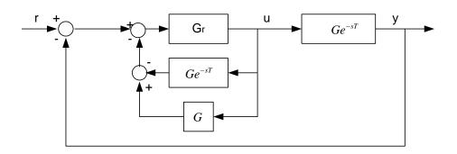
**Problem 4.** Consider the IMC control structure, which is used to control a stable and minimum phase SISO process G.
