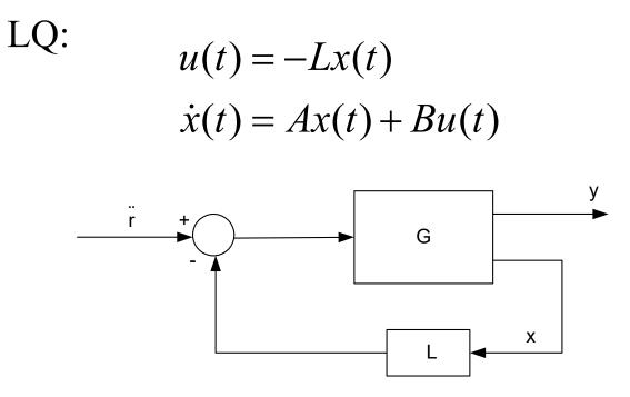
The loop transfer function (gain in control signal)
