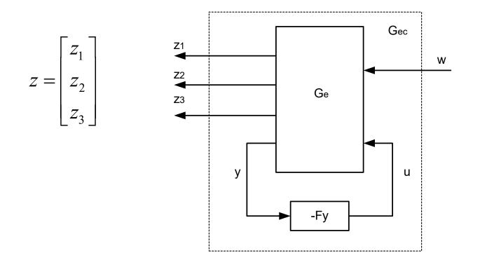
Generalized control configuration. When the control loop is closed, the transfer function from *w* to *z* is obtained.
