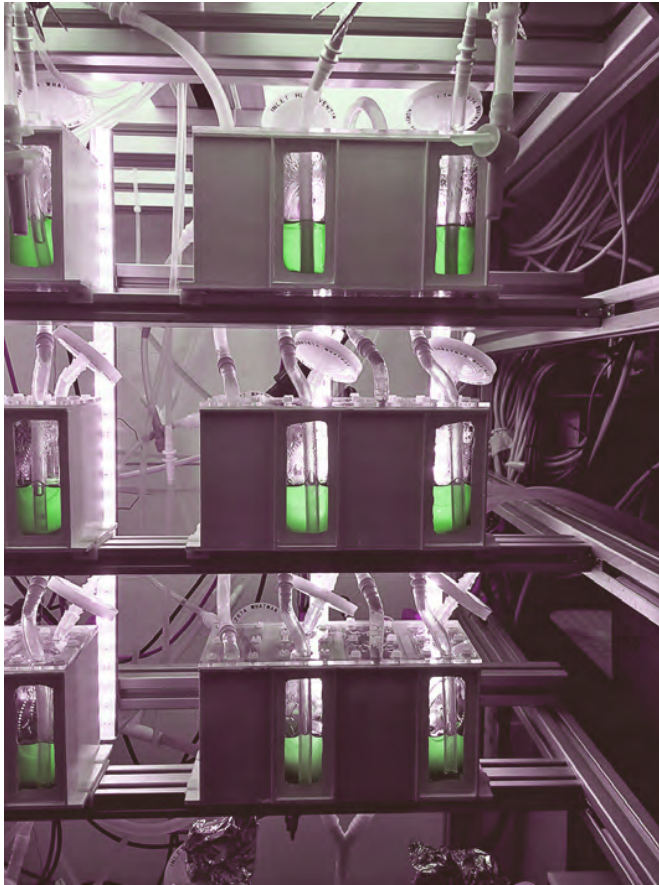
Fig. 2: Detail of the fully inoculated Living Architecture 'wall' and apparatus installed at the University of the West of England, Bristol. Photograph courtesy of Rachel Armstrong, the 'Living Architecture' project, 2019. © Rolf Hughes. A section of a bioreactor array showing three stacked units within the 'living' wall that houses microbes in a large apparatus about the size of a bookcase.
