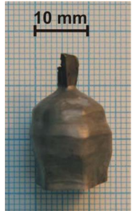
13 gram single crystal of \text{Ba}_8\text{Ga}_{16}\text{Ge}_{30} (Christensen et al. Nature Mater. 2008 , 7, 811)
