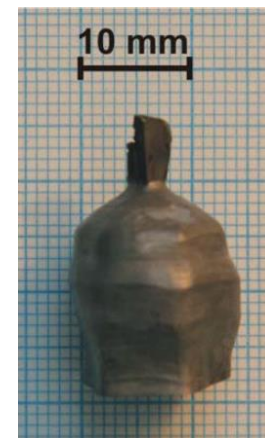
13 gram single crystal of \text{Ba}_8\text{Ga}_{16}\text{Ge}_{30} (Christensen et al. Nature Mater. 2008 , 7, 811)
