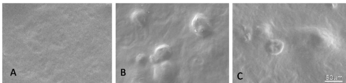
Fig. 7. Surface SEM images of starch film (A: pure starch film; B: containing starch crystals; C: containing cellulos crystals) [Reproduced from Ref. [90] with permission].
