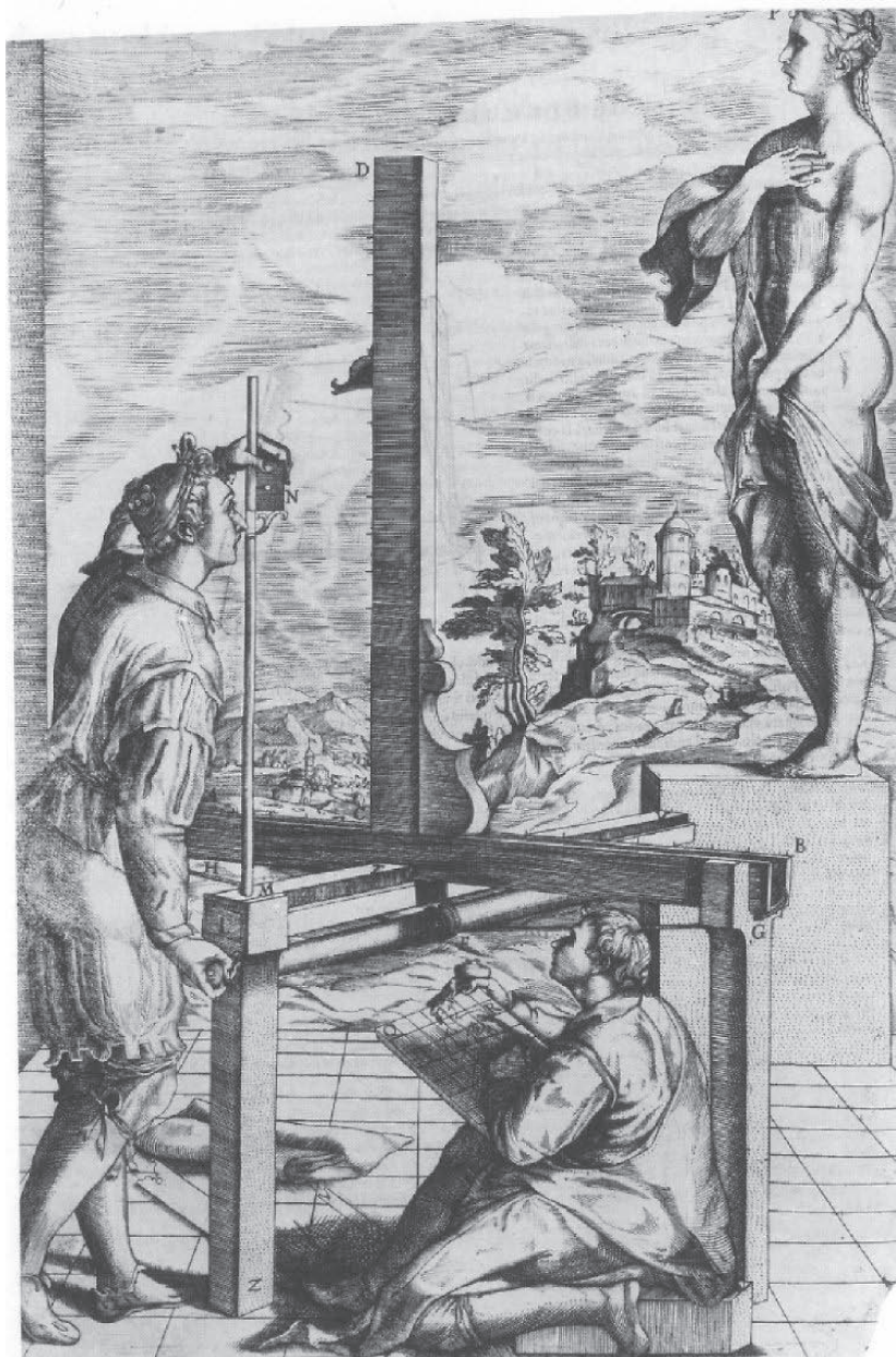
FIGURE 6-1. Achieving perspective without the velum . Notice the adlatus on the floor, holding the grid in his hands, on which he enters the coordinates the artist-engineer is telling him. Engraving, reprinted from Jacopo Barozzi da Vignola, Le due regole della prospettiva pratica (Rome: Stamparia Camerale, 1611).
