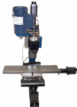
Figure 1: From left: a user-designed highlight is converted to an optimized microfacet height field. A computer-controlled milling machine is used to manufacture the surface ( 30 \times 30 facets, each approximately 1 \text{ mm} \times 1 \text{ mm} ), which exhibits the desired reflectance.
