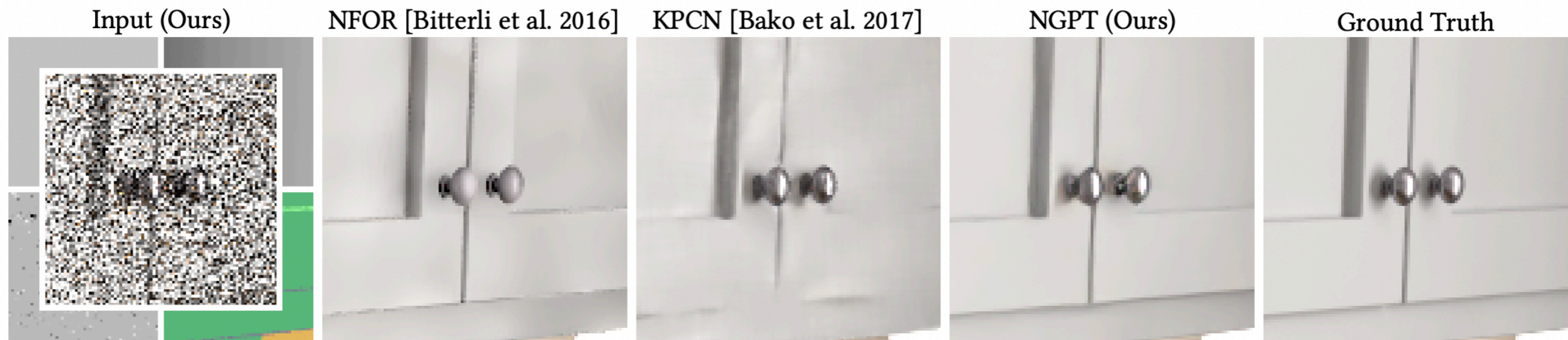
Fig. 1. Comparison of the primal-domain denoisers NFOR [Bitterli et al. 2016] and KPCN [Bako et al. 2017] to our gradient-domain reconstruction NGPT from very noisy equal-time inputs (8 samples for ours and 20 for others). Generally outperforming the comparison methods, our results show that gradient sampling is useful also in the context of non-linear neural image reconstruction, often resolving e.g. shadows better than techniques that do not make use of gradients.
