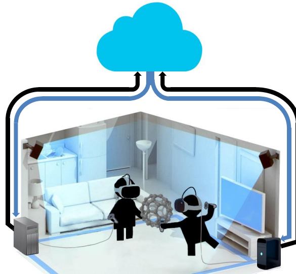
Figure 3: Multi-person VR framework setup in which bodies are co-present in the same space. This particular figure shows two people passing between themselves a simulated molecular object
