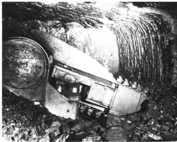
Figure 28. Dosco continuous miner in action.
