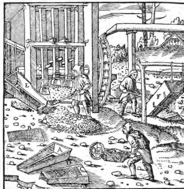
A—IRON LAID FLAT ON THE GROUND. B—ITS BOTTOM WHICH IS MADE OF IRON WIRE. C—BOX INVERTED. D—IRON RODS. E—BOX SUSPENDED FROM A BEAM, THE INSIDE BEING VISIBLE. F—BOX SUSPENDED FROM A BEAM, THE OUTSIDE BEING VISIBLE.
