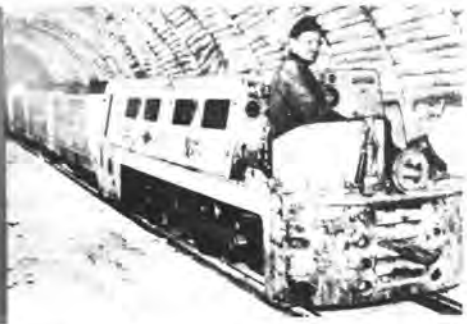
Typical of the "mechanical monsters" which have turned "Fiber" and "Steel" into "Coal" is this modern mode of underground transport — 100 H.P. Diesel Locomotive, operated by the Mines Trading Station, Buxton, England, for use underground in coal mines. Thirty of these locomotives are in use in the Cape Breton, Nova Scotia, mines of the Dominion Coal Company, Limited. The introduction of these locomotives to increase transportation efficiency underground is part of Devco's extensive mines mechanization programme.
