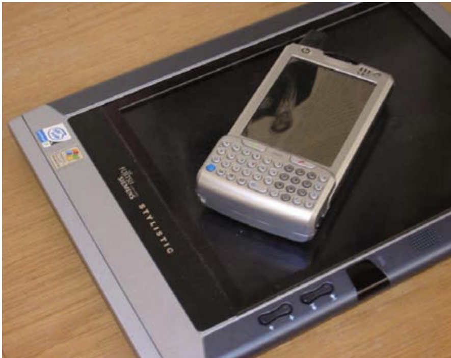
Figure 24.4.: A Tablet PC with a touch display and a personal digital assistant (PDA) with a resistive screen.
