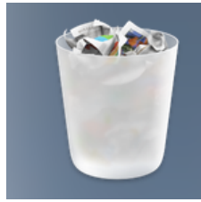
Figure 28.4.: An example a commonplace metaphor in GUI desktops: the bin as a representation of deleting files. This is the Mac OS X bin. Users can delete files by dragging them to the bin (or issuing a delete command directly). By clicking the bin the file management application shows the user previously deleted files, which can then be recovered if the user so chooses.
