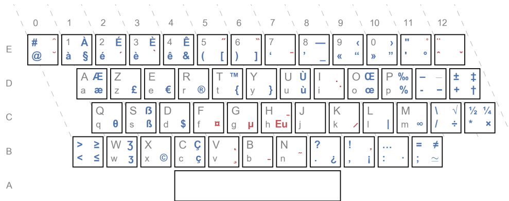
Figure 39.9.: The new Azerty standard was designed with the help of multi-objective optimization [235].
