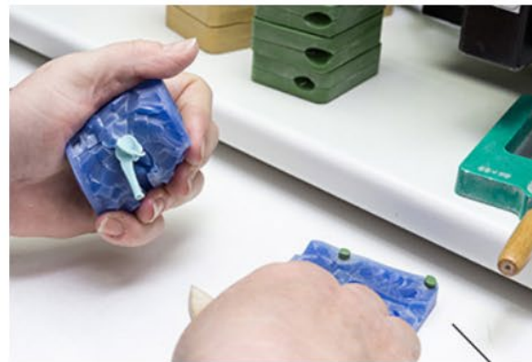
Some of the wax models are still created traditionally by hand. Hot wax is injected inside a rubber mold and the solidified wax model is carefully removed from the mold.
