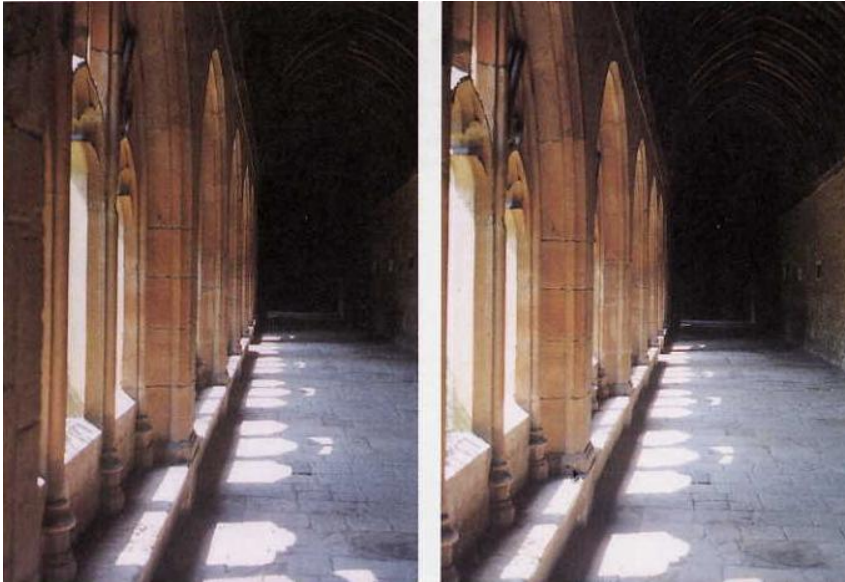
Stereopair of the Cloisters, New College, Oxford. The right photograph was taken, the camera was shifted about 3 inches to the left, and the left photograph was taken.
