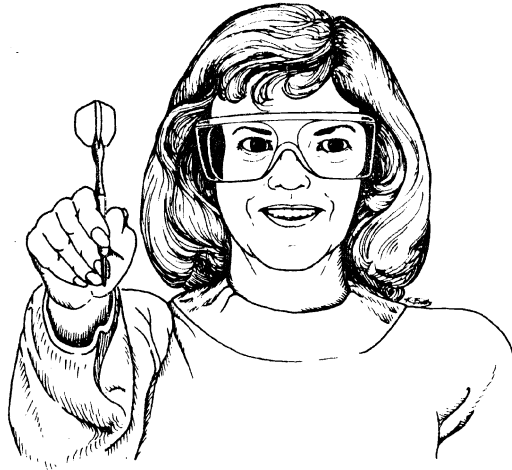
Figure 7.1. Throwing darts while wearing wedge prism spectacles (base to the right). The subject is looking directly at the target toward which she is pointing the dart, but because the prism bends the optic path 15 degrees to the right, her gaze is deviated 15 degrees to her left to see the target (she is looking at you). The portion of her face behind the lenses appears to the viewer to be displaced to her left because of the prism's bending of the optic path. The direction of throw is normally in the direction of gaze. The gaze direction has, however, been calibrated to the throw direction, and the aim of throw is true (at you). (From Thach, Goodkin, and Keating 1992; in Annual Review of Neuroscience , Volume 15, copyright 1992, Annual Reviews [www.AnnualReviews.org]; reprinted by permission from publisher and author.)
