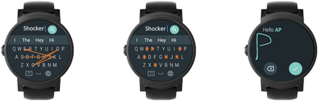
Figure 1. Google keyboard with trace input (left), Google keyboard with standard point-and-tap input (middle), and Google Handwriting Input app (right).
