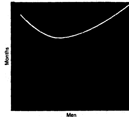
Fig. 3. Since software construction is complex, the communications overhead is great. Adding more men can lengthen, rather than shorten, the schedule.
