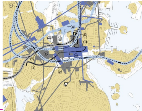
Underground facilities and space reservations in center of Helsinki. City of Helsinki,
