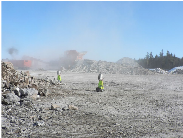
Measurement at downwind distances 40 m and 50 m from the crusher (Sairanen et al 2017)
