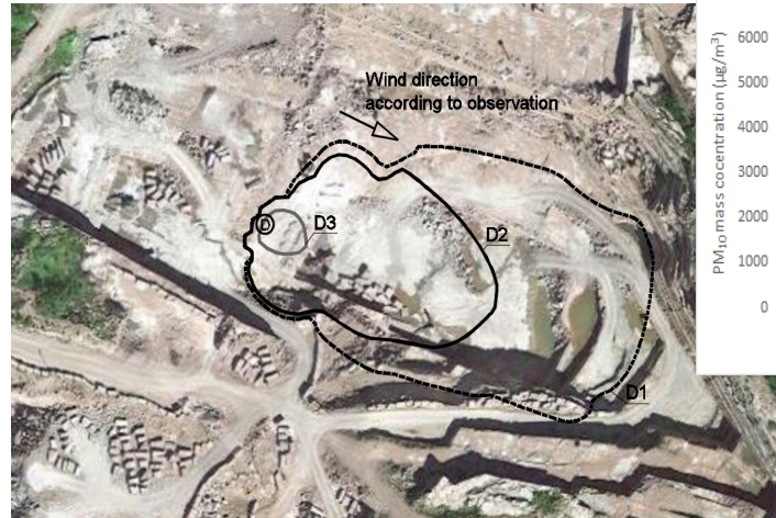
Predicted concentration contours ( 50 \mu\text{g PM}_{10}/\text{m}^3 ) according to three models (M. Sairanen, unpublished).
