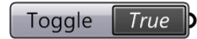
Boolean Toggle - double click the boolean value to toggle between true and false
