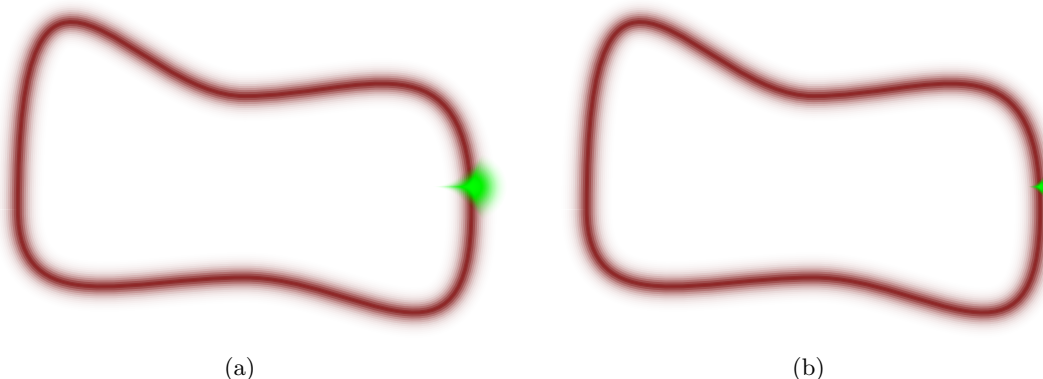
FIG 10. In high dimensions, the Random Walk Metropolis proposal density (green) is strongly biased towards the outside of the typical set where the target density, and hence the Metropolis acceptance probability vanishes. (a) If the proposal variances are large then the proposals will stray too far away from the typical set and are rejected. (b) Smaller proposal variances stay within the typical set and hence are accepted, but the resulting transition density concentrates tightly around the initial point. Either way we end up with a Markov chain that explores the typical set very, very slowly.
