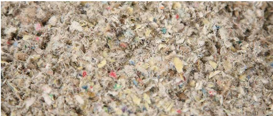
Figure 13. Cellulose Insulation.
