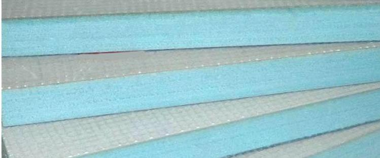
Figure 11. Extruded Polystyrene (XPS)
