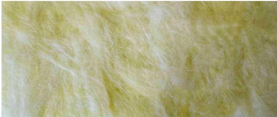
Figure 6. Glass mineral wool insulation
