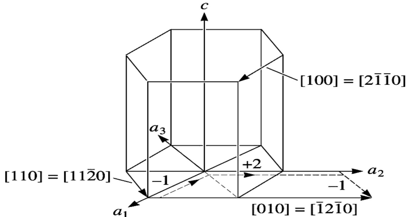
Typical directions in the hexagonal unit cell, using both three- and four-axis systems. The dashed lines show that the  $[\bar{1}2\bar{1}0]$  direction is equivalent to a  $[010]$  direction.
