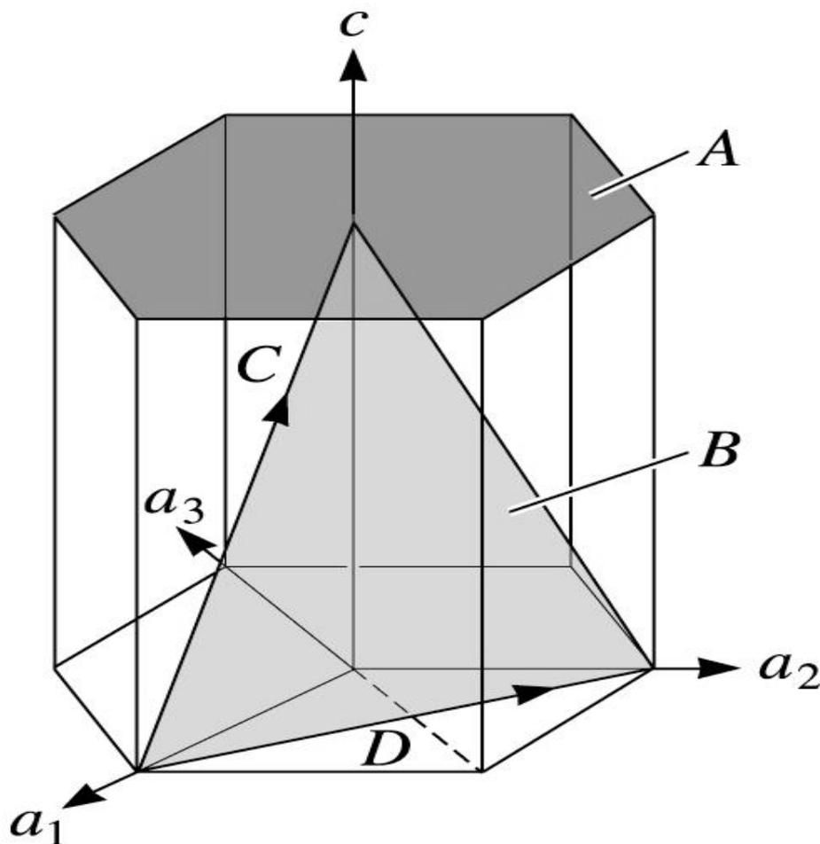
Miller-Bravais indices are obtained for crystallographic planes, directions, and points in hexagonal unit cells by using a **four-axis coordinate system**.
