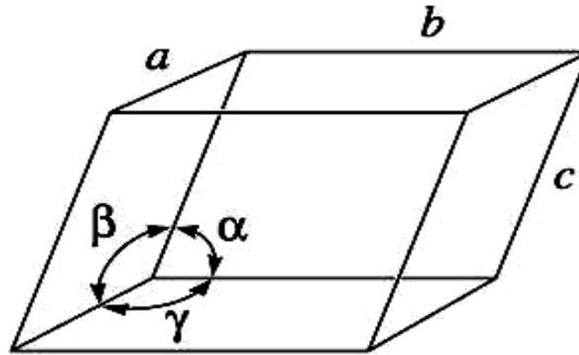
**Definition of lattice parameters in cubic, orthorhombic, and hexagonal crystal systems.**
