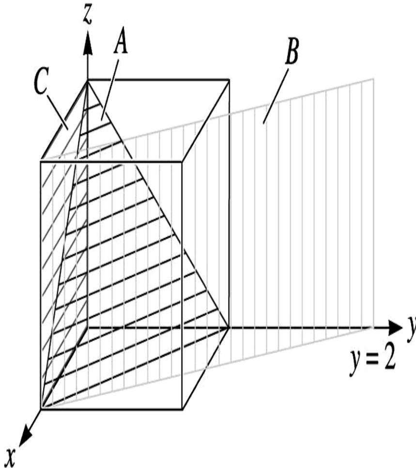
Identify the coordinate intercepts of the plane, if plane is parallel to one of the axes, this intercept is taken to be infinite
