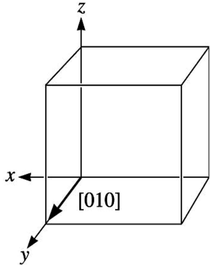
Equivalency of crystallographic directions of a form in cubic systems.
