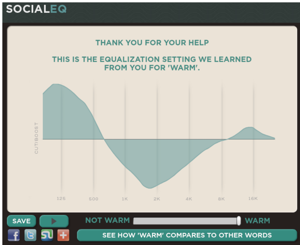
Figure 8: End result of a short session with SocialEQ.org, trying to define what a warm sound is like. The user interface allows the user to save the processed file, to play back the filtered sound and to morph the filter between the original and its inverse.
