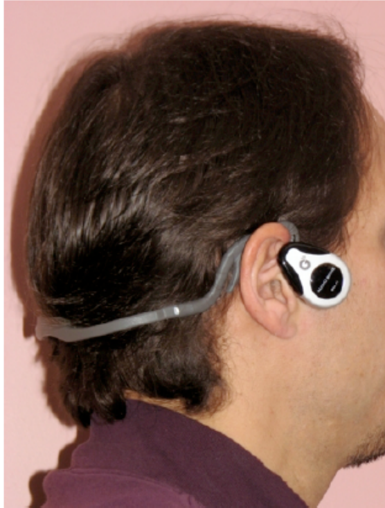
Figure 11: Bone conducting headset used in test in [14] [15].
