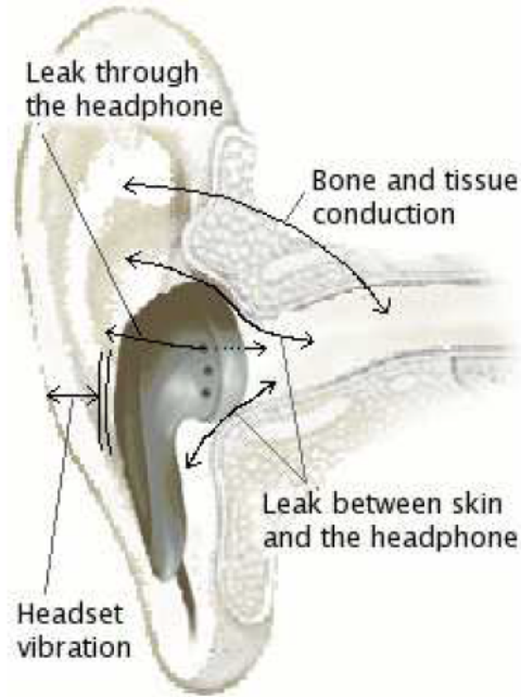
Figure 8: Different ways sound leaks when wearing headphones [32].
