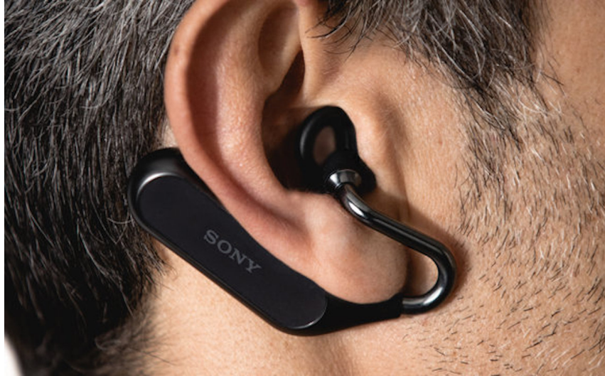
Figure 5: Commercially available ARA headset [21] that does not block the ear canal entirely.
