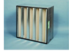
Figure 3.10 Example of HEPA and ULPA filters. The panel type (left) is mainly used for unidirectional (previously called laminar) flows in clean rooms or clean benches at a face velocity of 0.45 m/s. The compact type (right) is used for inlet or exhaust air system with high air flows, up to 3 m/s face velocity.
