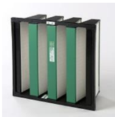
Figure 3.9 Examples of fine filters. The compact filters are made of thin (~ 0.5 mm) and stiff pleated filter material of glass or polymer.
