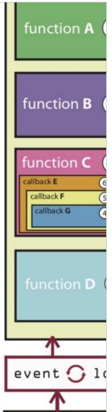
When we offload IO to a separate thread with the browser API, we need to somehow get the reply back. That's what the event queue is for. The difference is how we do it conveniently and also handle errors.
