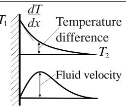
Free convection from a warm surface  $(T_1 > T_2)$
