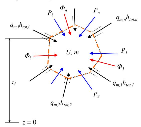
Enthalpy flow Mechanical power Heat flow System boundary Energy balance:  $\sum_{i} P_i + \sum_{i} \Phi_i + \sum_{i} q_{m,i} h_{tot,i} = \frac{dU}{dt}$ Mass balance:  $\sum_{i} q_{m,i} = \frac{dm}{dt}$
