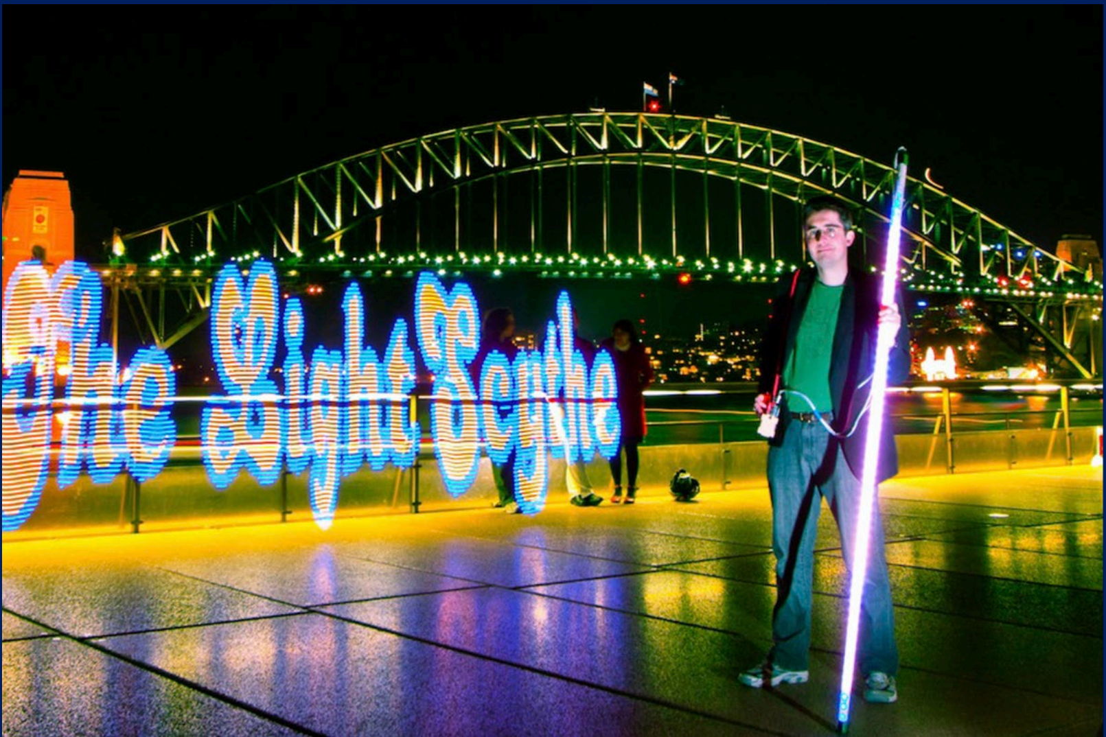
Figure 3.22. This image shows 'LightScythe', an open-source wand-based light painting tool inspired by Immaterials: Light Painting WiFi . The tool, and the instructions for how to make one, were created by a man who calls himself 'The Mechatronics Guy': https://sites.google.com/site/mechatronicsguy/lightscythe . Credit: 'The Mechatronics Guy'.
