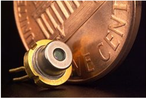
A packaged laser diode with penny for scale
