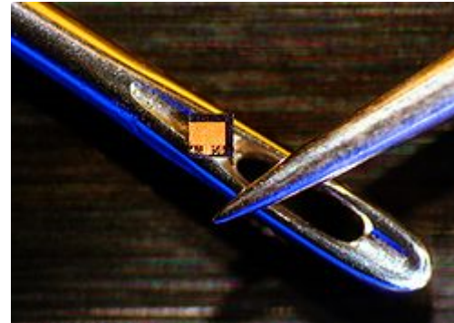
Image of the actual laser diode chip (shown on the eye of a needle for scale) contained within the package shown in the left image.
