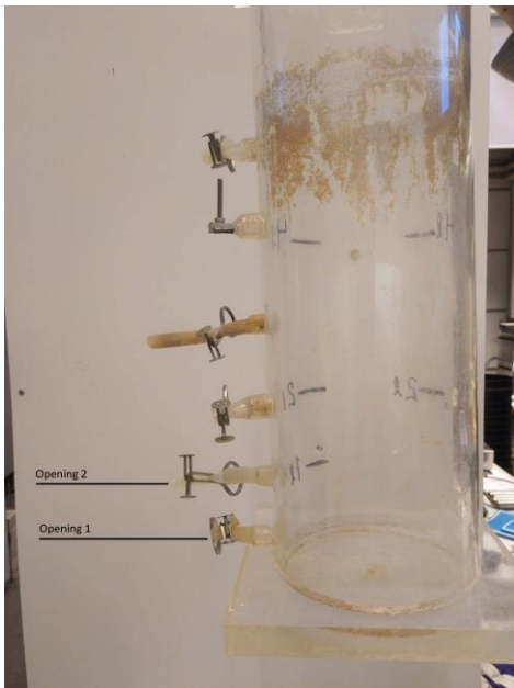
Figure 6. Column for DAF tests. Air is added from opening 1, and samples can be taken from opening 2 to assess water quality.
