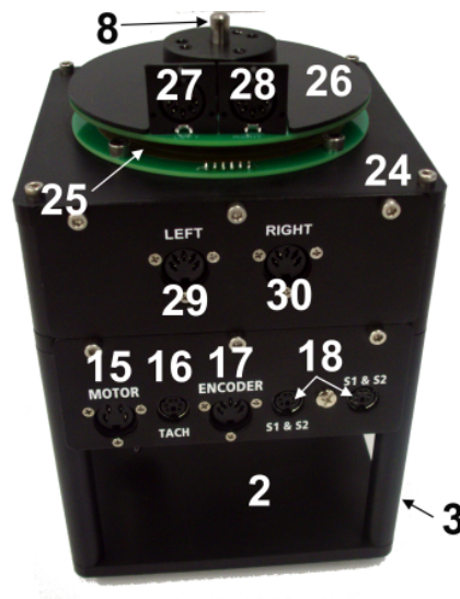
Figure 2.6: Components on the SRV02-ETS
