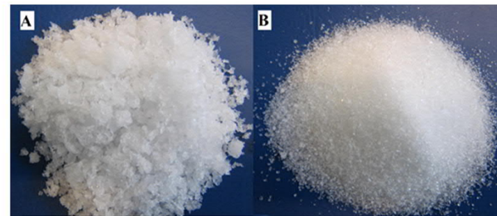
Figure 1. (A) (\text{NH}_4)_2\text{SO}_4 produced by NHT, (B) commercial (\text{NH}_4)_2\text{SO}_4
