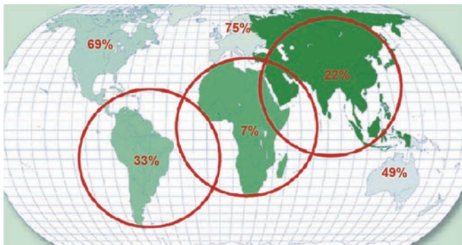
Fig. 2. Hydropower undeveloped technical potential.
