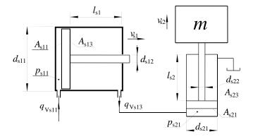
**E**. Calculate the pressure  $p_{s11}$  required for lifting the load (system assumed to be ideal; no losses).
