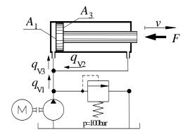
Selecting the piston areas to fulfill criteria  $A_1 = 2 \cdot A_3$ will result in equal piston velocities in both directions when connections for outward stroke are as in case 3 and for inward stroke as in case 2. One possible implementation of such system adjacent.
