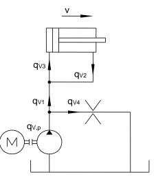
$$q_{V1} = q_{V3} - q_{V2} = (0.0015 - 0.001) \frac{\text{m}^3}{\text{s}} = 0.0005 \frac{\text{m}^3}{\text{s}} = 30 \frac{1}{\text{min}}$$
