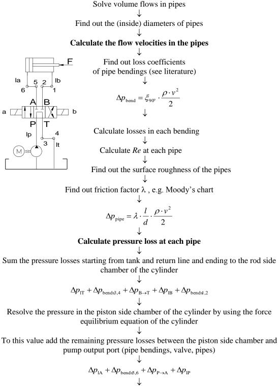
The pressure at the pump outlet port  $p_p$  is resolved!
