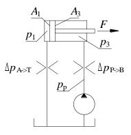
$p_{\rm p} = p_3 + \Delta p_{\rm P \to B} = 13.2 \text{MPa} + 0.8 \text{MPa} = 14 \text{MPa}$
