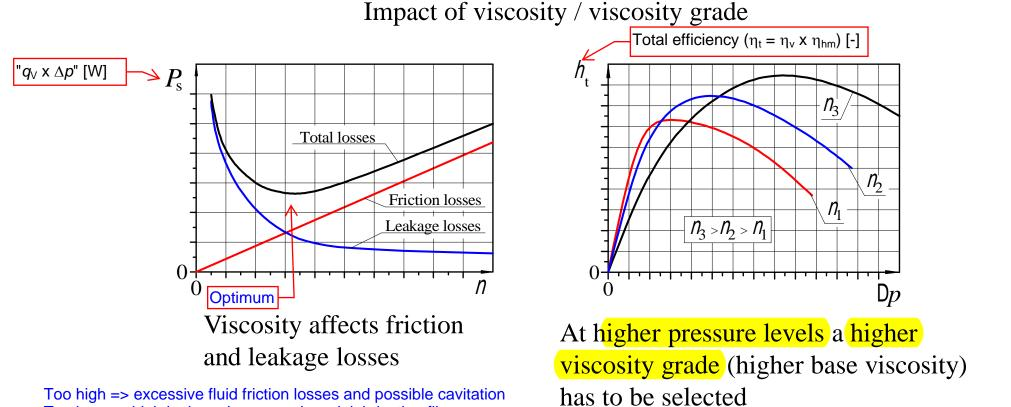
Too high => excessive fluid friction losses and possible cavitation Too low => high leakage losses and weak lubrication film
